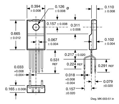
**Dimensions in Millimeters** (controlling dimensions)
