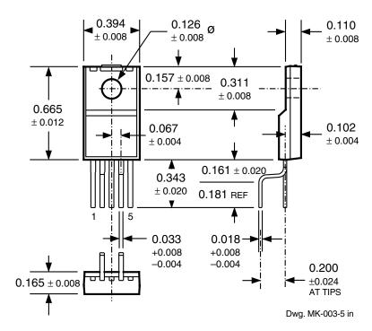
Dimensions in Millimeters (controlling dimensions)
